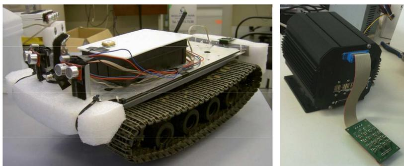
The embedded platform is capable of running the IQR neural network simulator, doing sensor read-out and even controlling a mobile robot.
