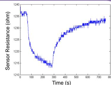
Single sensor response to 4ppm of ammonia. Response time ( $t_{90\%}$ ) = 90s
