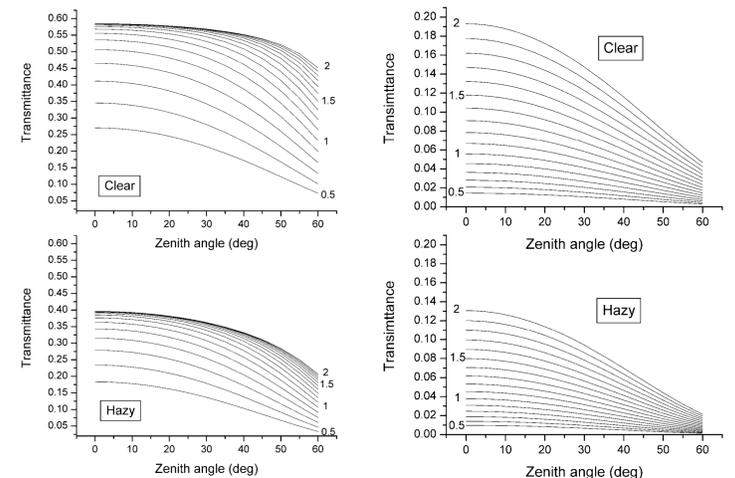
Figure 4. Superdense coding, Transmittances in space-Earth communication (downlink left, uplink right) at various seasons, latitudes and weather conditions. Labels over the graphs indicate Bob's detector diameter in meters. Alice's aperture size is fixed as 0.2, the satellite is orbiting at 300 km.
