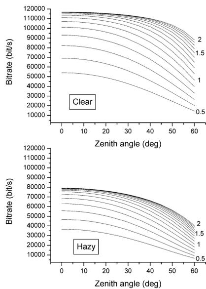
Figure 2. Bitrates of BB84 secure key generation rate in space-Earth communication at various seasons, latitudes and weather conditions. Labels over the graphs indicate Bob's detector diameter in meters. The laser pulses are generated at a 1 MHz rate.
