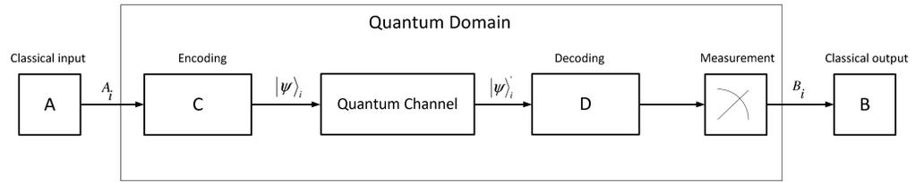
Figure 1. Transmission of classical information through the satellite quantum channel. We encode the classical information into a quantum bit, then we send the quantum bit over the quantum channel. At the end we have to decode and measure it to get back a classical information.
