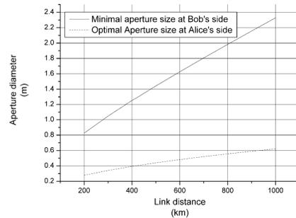
Figure 3. Superdense coding, optimal aperture size at Alice's side (at which the beam spreading is lowest) as the function of the link distance has been plotted by continuous line. Dashed line represents minimal aperture diameter at Bob's side for the protocol to be worthwhile.
